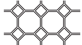
10" Diamond Tile Tile Size 262 x 262mm, Diamond Size 100 x 100mm
